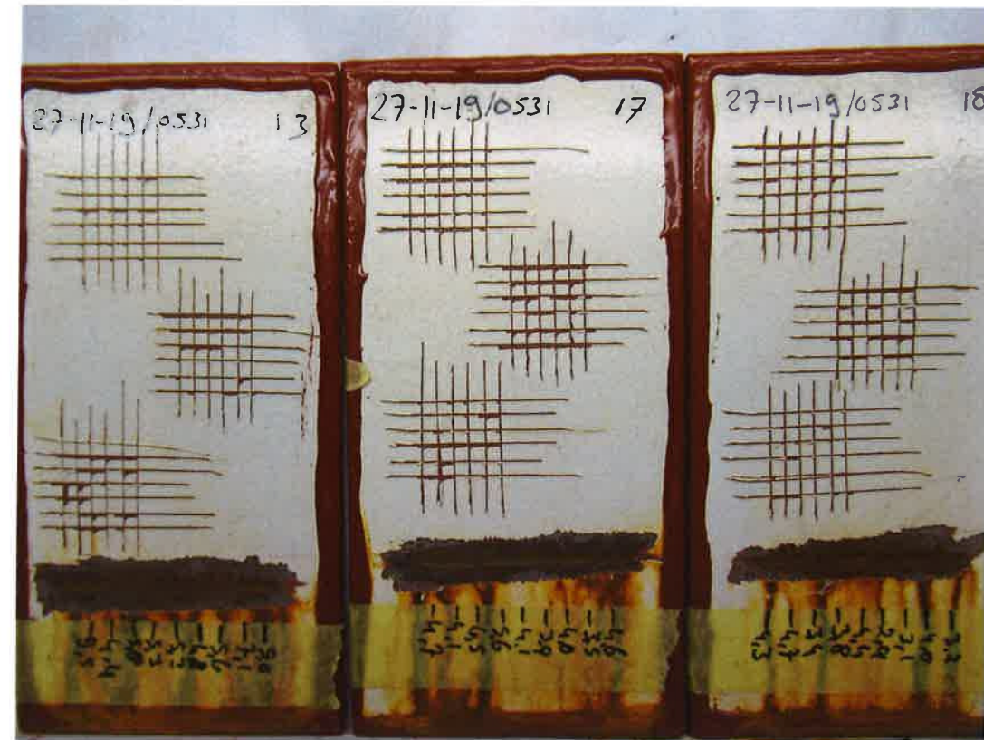
Photo 2: Panels 13, 17 and 18 after 1440 hours Neutral Salt Spray test.
