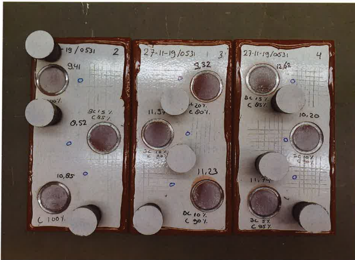
Photo 1: Panels 2, 3 and 4 Reference adhesion
