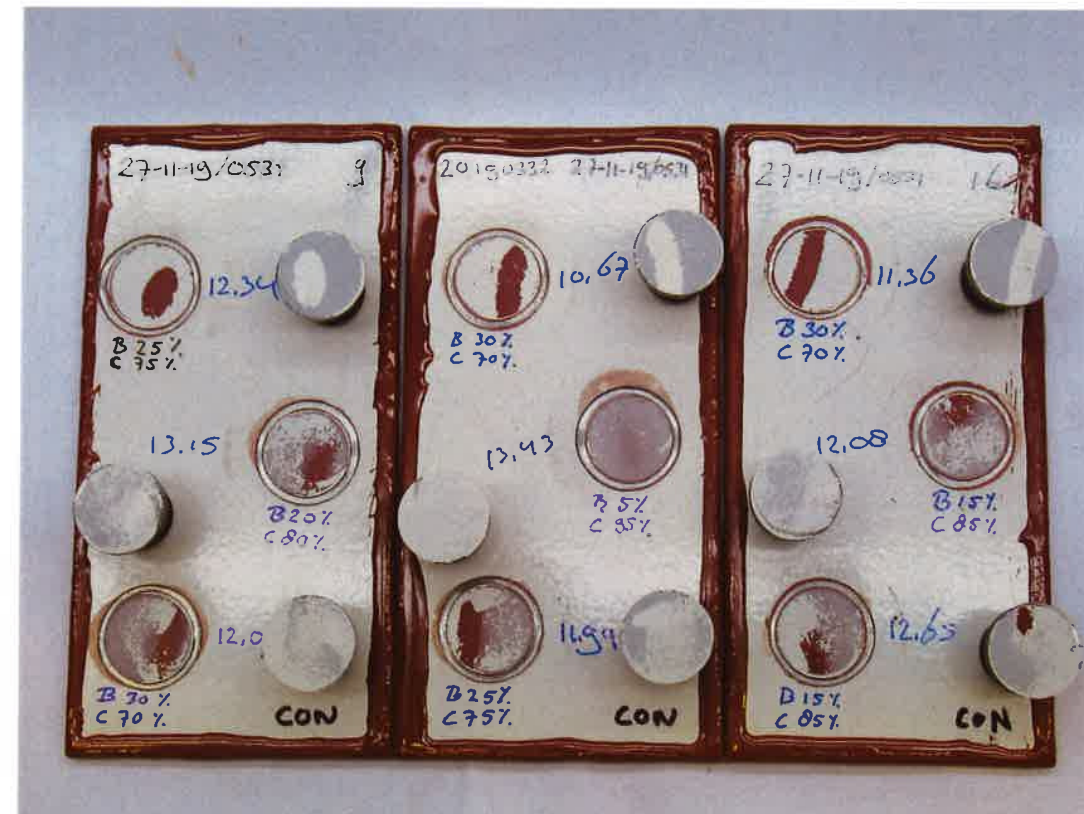
Photo 3: Panels 9, 11 and 16 after 720 hours Water Condensation test.
